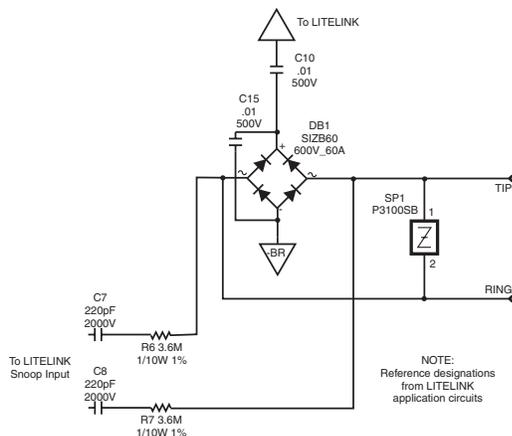
Note the surge protection block across the tip and ring leads in Figure 2. This device is normally specified to clamp surge voltages in excess of the maximum ring voltage between tip and ring (metallic surge protection).
