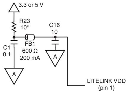
With particularly noisy power supplies, substitute an inductor for R23. IXYS IC Division recommends a value of 220 $\mu$ H in this application, Toko 380HB-2215 or similar.
