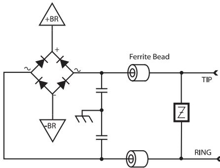
Figure 3 shows an EMI filter that can be applied to LITELINK circuits in conjunction with the standard application circuit in systems using Earth ground. This circuit helps prevent coupling host device emissions to the telephone line.
